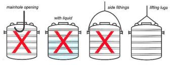
STRICTLY Lifted / unloaded at at lifting lugs provided.
